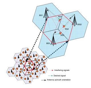
Fig. 2. A pictorial illustration of how system wide optimization of tilts can be decomposed into optimization of tilts within each triplet independently.
