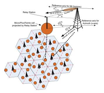
Fig. 1. System model for problem formulation. Small circles show location of Relay Stations based cells within each sector (macro cell).
