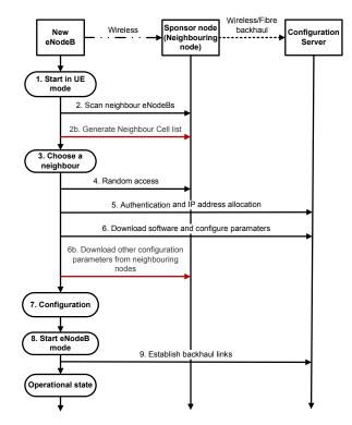
Fig. 4. Self Configuration Flow Chart
