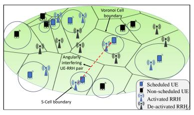
Fig. 1: The UE-centric S-cell architecture. The Voronoi tessellation of the plane is formed by  $\Phi_{UE}$ . The circles around UEs represent S-cell edges at  $\zeta = 1/2$ . S-cell boundaries are not drawn to scale.
