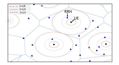
Fig. 2: The UE-centric Stienen cell sizes with different  $\zeta$  values.
