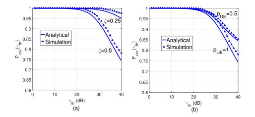
Fig. 3: SINR coverage probability at: (a) different  $\zeta$  and  $p_{\text{UE}}=1$ , (b) different  $p_{\text{UE}}$  and  $\zeta = 0.5$ .
