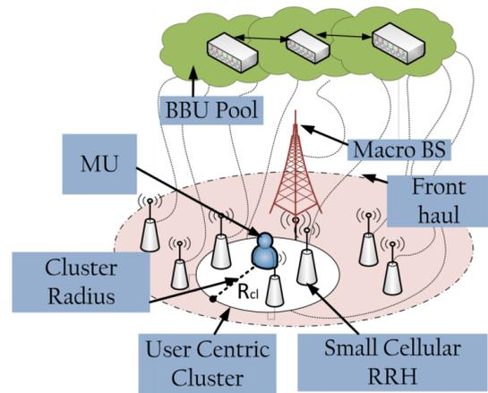
**FIGURE 1.** UC-RAN architecture with activation disc of radius  $R_{cl}$  for a served user.
