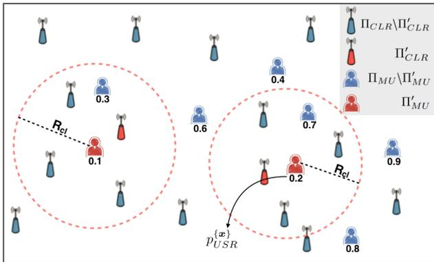
**FIGURE 2.** User-centric RRH clustering in a UC-RAN. Each scheduled user is served by a single RRH in its respective cluster that maximizes its received SIR. The user-centric scheduling is based on  $p_{USR}^{(x)}$  values with lower marks corresponding to high scheduling priorities.
