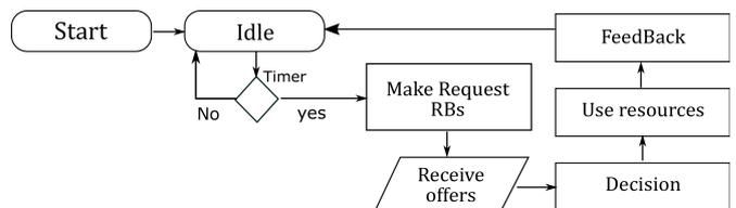
Fig. 2: User equipment flowchart: Service request and usage.
