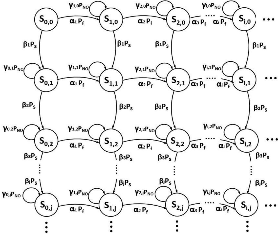
Fig. 5. Markov chain modeling of no-handover, handover failure and handover success related core-network mobility signalling.
