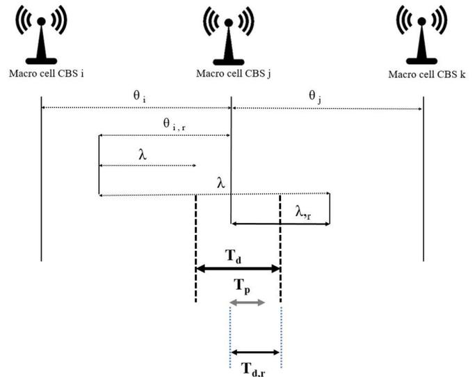
Fig. 3. Timing diagram of handover model parameters.
