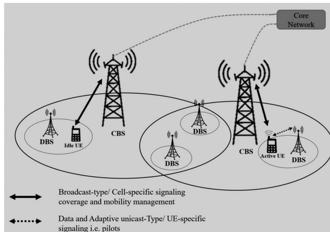
Fig. 2. Schematic of control data plane separated Architecture.
