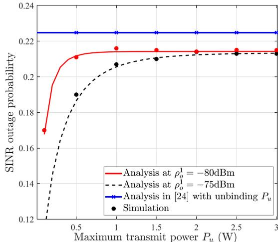
Fig. 3. Effect of the maximum transmit power in a single-tier mmWave network for  $\theta_1 = 20$  dB,  $\beta_1 = 0.0071$ ,  $\alpha_L^1 = 2$ ,  $\alpha_N^1 = 4$ , and BS densities  $\lambda = 10$  BS/km<sup>2</sup>.
