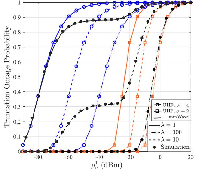
Fig. 8. Comparison of the truncation outage probability of mmWave and UHF cellular networks for BS density  $\lambda = 1, 10$ , and  $100$  BS/km<sup>2</sup>.  $\beta_1 = 0.0071$ ,  $\alpha_L^1 = 2$ , and  $\alpha_N^1 = 4$  in the mmWave network.
