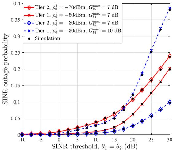
Fig. 2. Comparison of the analytical results with simulation in a two-tier mmWave network for  $\beta_1 = 0.0071$ ,  $\beta_2 = 0.0143$ ,  $\alpha_L^1 = 2$ ,  $\alpha_N^1 = 4$ ,  $\alpha_L^2 = 2.9$ , and  $\alpha_N^2 = 5$ , and BS densities  $\lambda_1 = 10$  BS/km<sup>2</sup> and  $\lambda_2 = 2\lambda_1$ . Red and blue dashed-lines represent mmWave networks 1 and 2, respectively.
