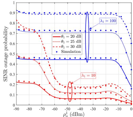
Fig. 4. Effect of the BS density on the SINR outage probability for  $\lambda_1 = 10$  and  $100$  BS/km<sup>2</sup>,  $\beta_1 = 0.0071$ ,  $\alpha_L^1 = 2$ , and  $\alpha_N^1 = 4$  in a single-tier network.
