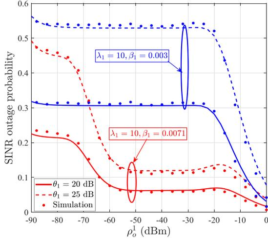
Fig. 5. Effect of the blockage parameter on the SINR outage probability for  $\beta_1 = 0.0071$  and  $0.003$ ,  $\lambda_1 = 10$  BS/km<sup>2</sup>,  $\alpha_L^1 = 2$ , and  $\alpha_N^1 = 4$  in a single-tier network.
