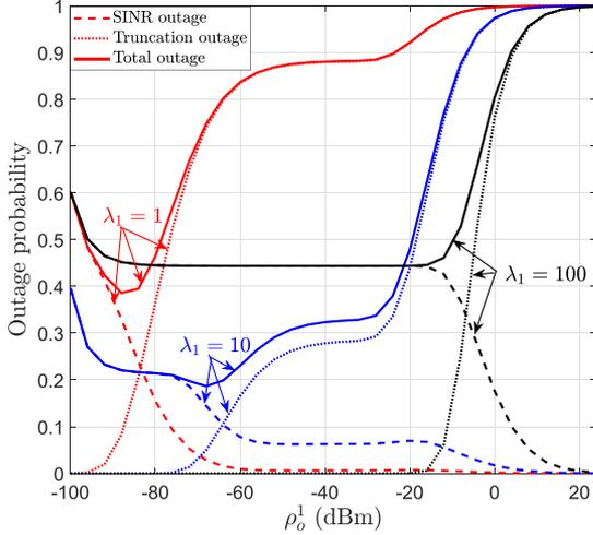
Fig. 9. Total outage probability in a single-tier mmWave network with  $\theta_1 = 20$  dB,  $\beta_1 = 0.0071$ ,  $\alpha_L^1 = 2$ ,  $\alpha_N^1 = 4$ , and BS density  $\lambda = 1, 10$ , and  $100$  BS/km<sup>2</sup>.
