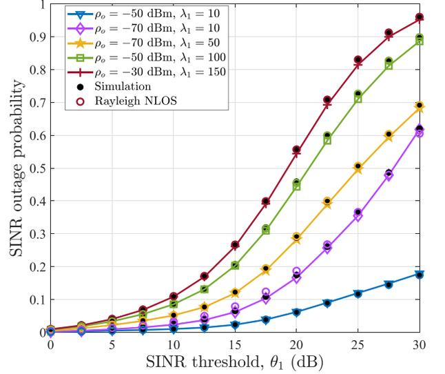
Fig. 1. Comparison of the analytical results with simulation in single-tier mmWave networks for  $\beta_1 = 0.0071$ ,  $\alpha_L^1 = 2$ , and  $\alpha_N^1 = 4$ .
