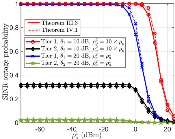
Fig. 7. Dense network approximation of the SINR outage probability in a two-tier mmWave network with  $\alpha_L^1 = 2$ ,  $\alpha_N^1 = 4$ ,  $\alpha_L^2 = 2.9$ ,  $\alpha_N^2 = 5$ ,  $R_B = 200$  m,  $\lambda_0 = 100$ ,  $\lambda_2 = 2\lambda_1$ ,  $G_{b1}^{\max} = 10$  dB, and  $G_{b2}^{\max} = 7$  dB.
