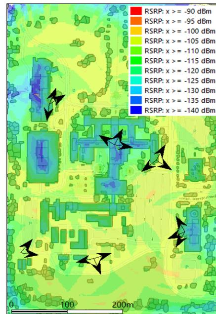
**FIGURE 4:** Optimized RSRP simulations using Atoll.
