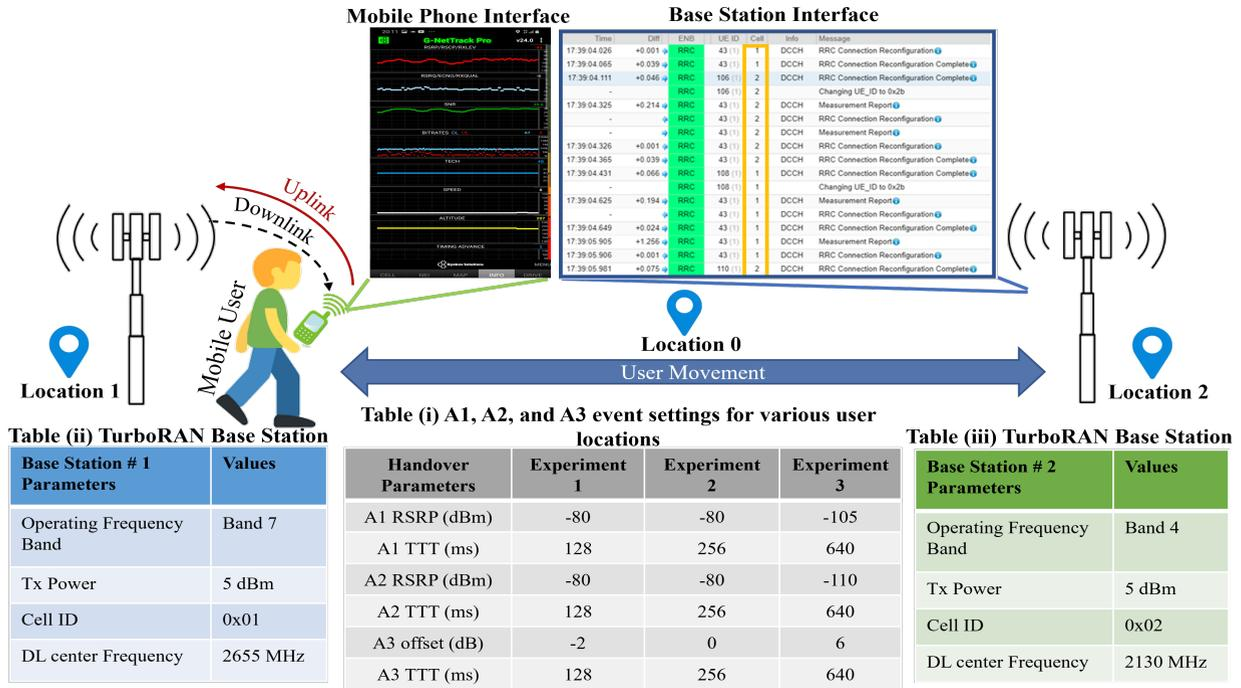
FIGURE 6: Inter-frequency handover use case experimental setup.
