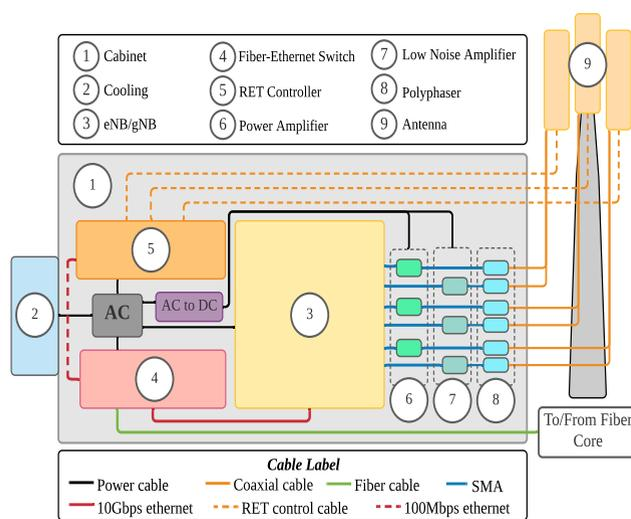
**FIGURE 3:** Block diagram representation of the TurboRAN testbed deployment.
