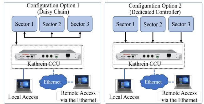
**FIGURE 5:** Two options for RET configurations.
